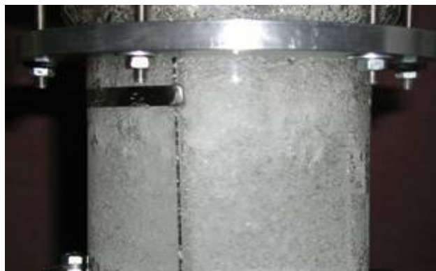
Figure 9. Gas-Liquid mixing. Air and water at 20 g acceleration.
