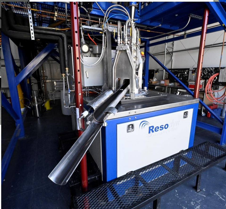
Two collection positions for in-spec and out of spec material
