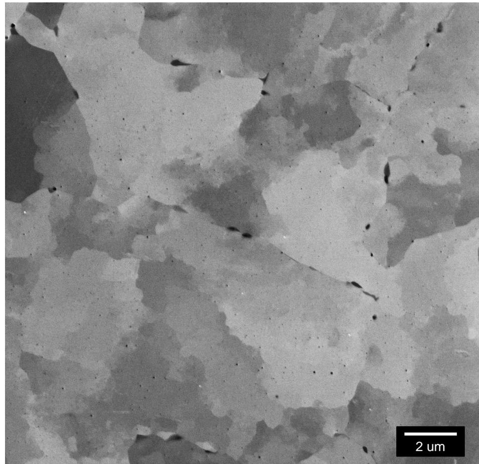
High resolution SEM reveals dispersed nano-oxides and grain boundary phases.
