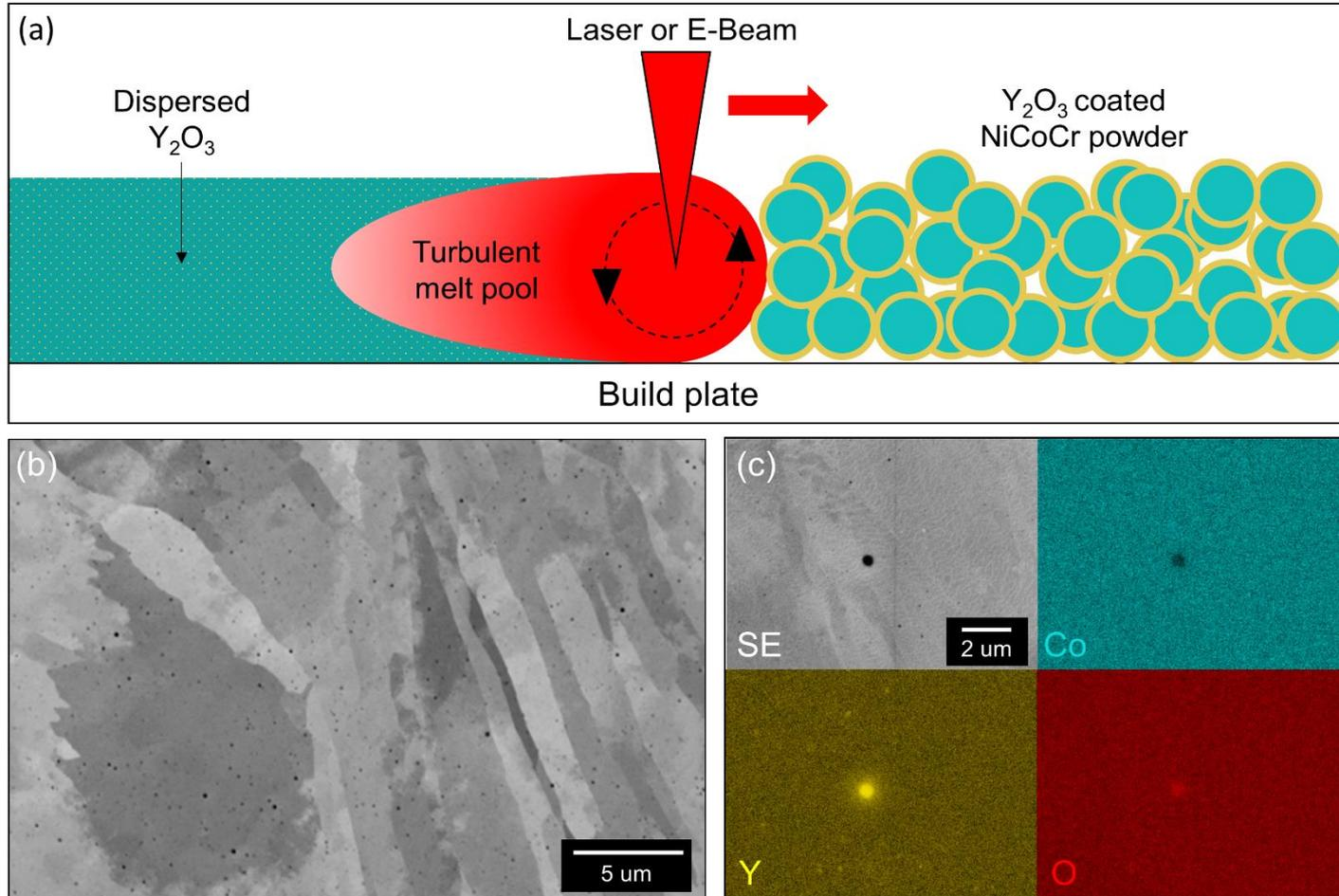
L-PBF successfully disperses the nano-scale  $Y_2O_3$  particles throughout the AM build
