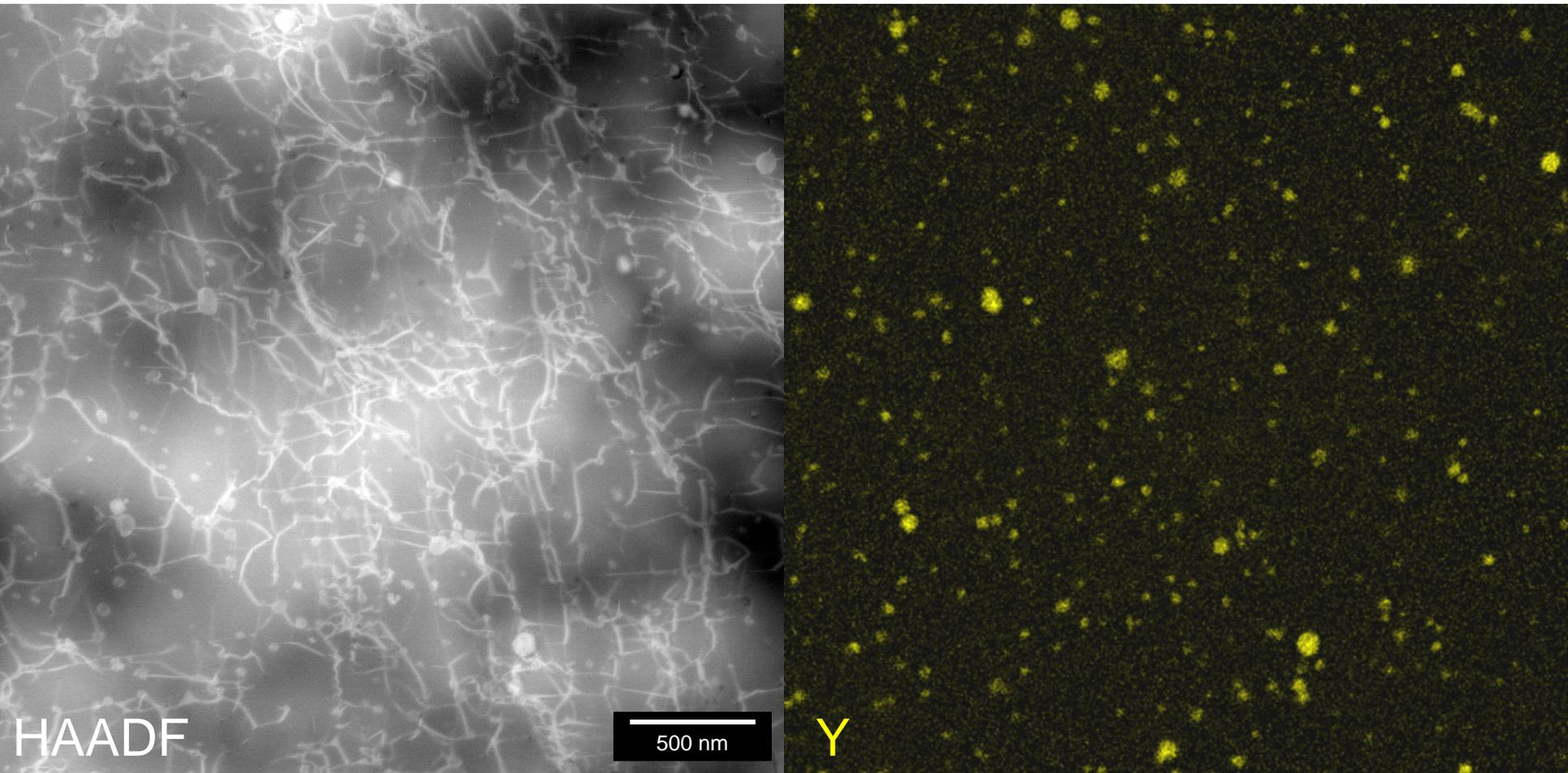
STEM-EDS analysis confirms high density of nano-scale  $Y_2O_3$  particles throughout bulk. No oxide agglomeration was present. Most other elements did not react with oxides (Nb and Ti were exceptions).
