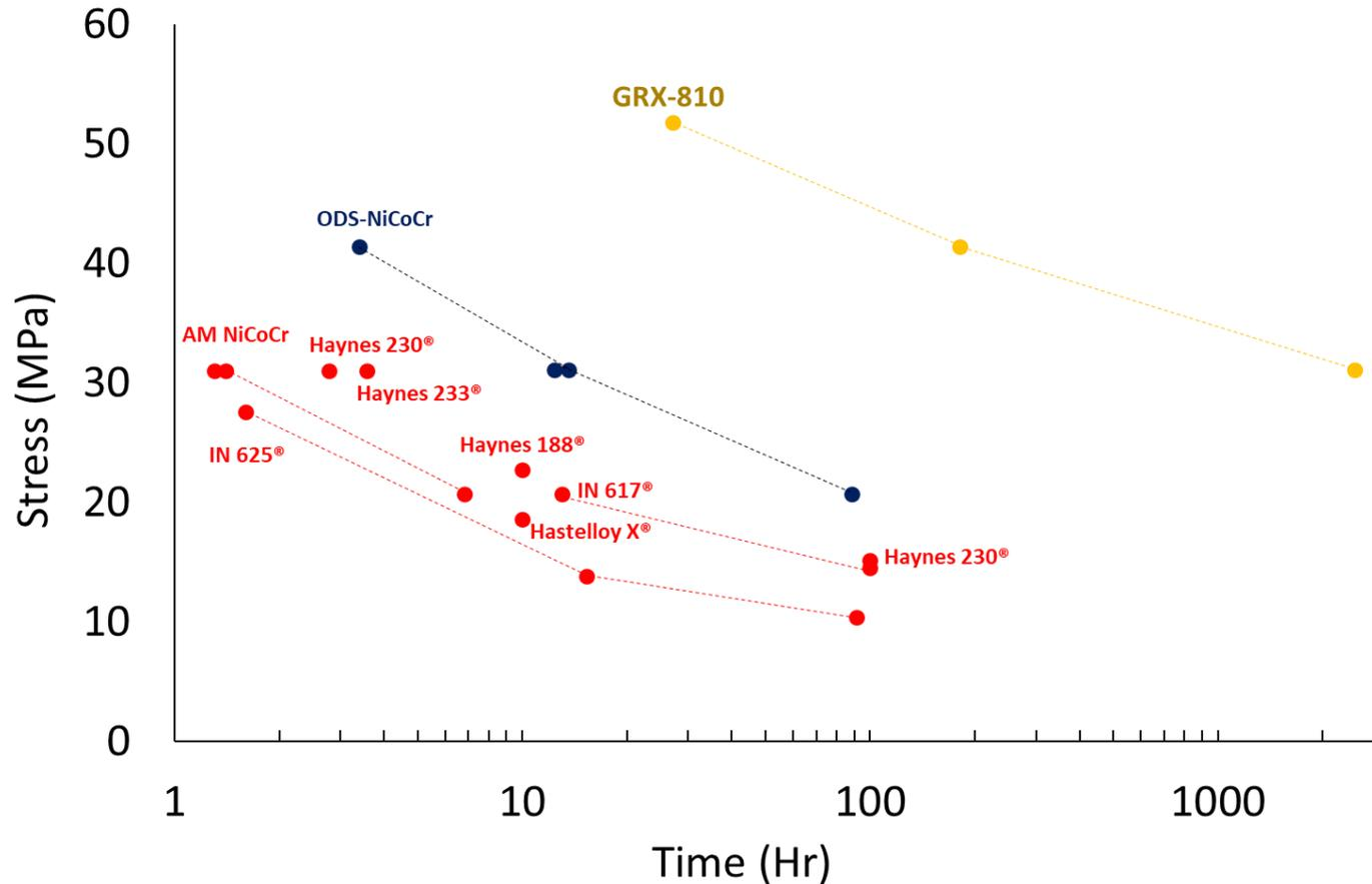
Alloy GRX-810 provides magnitudes of order better creep strength compared to conventional superalloys at 1093°C.
