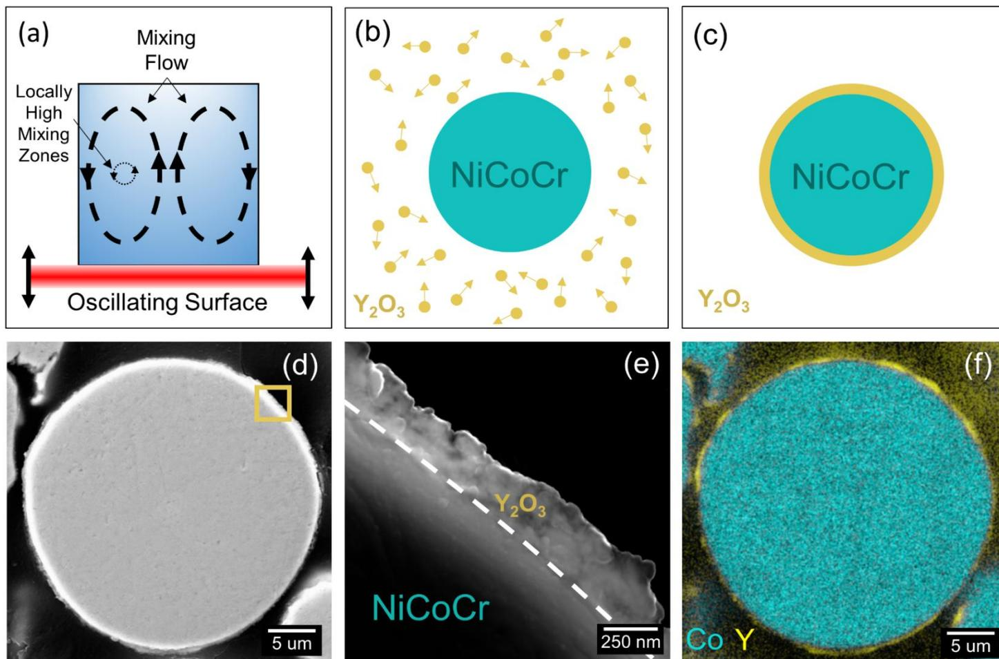
New high energy mixing technique successfully coats NiCoCr powder with 1 wt.% Y<sub>2</sub>O<sub>3</sub>.
