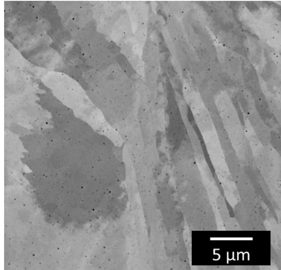
Nano-scale  $Y_2O_3$  particles are randomly dispersed throughout microstructure.
