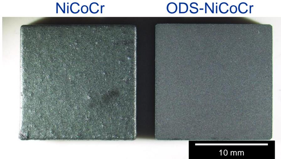
Left: Surface oxidation between NiCoCr and ODS-NiCoCr after 100hr-1100°C and 10hr-1200°C
