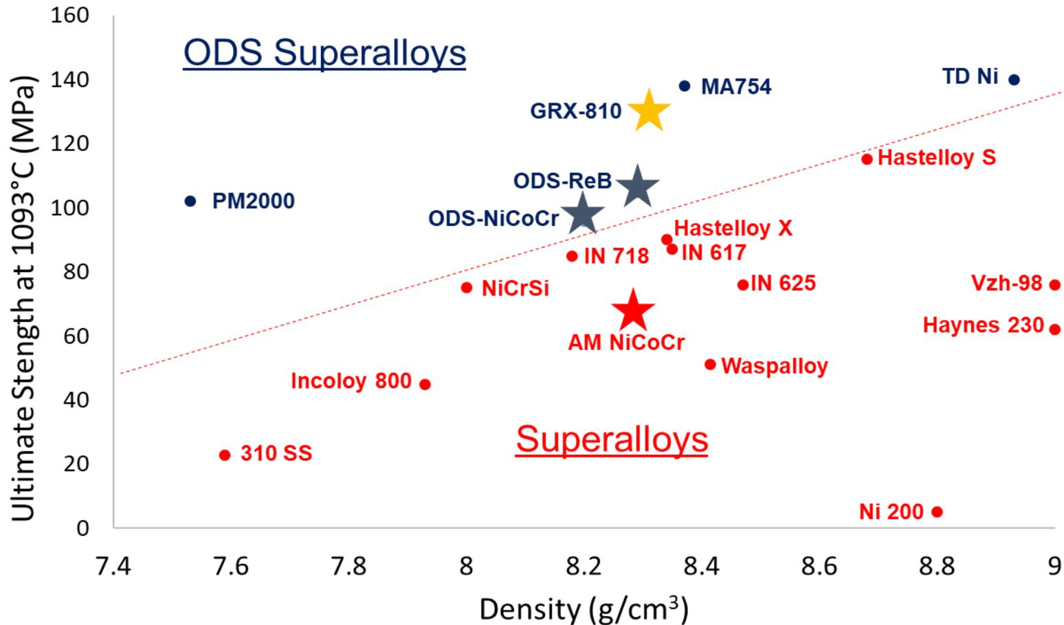
Scatter plot confirms the successful production of a ODS alloys using AM
