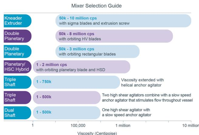
Figure 1. Viscosity limits of conventional mixers. Reproduced from [9].
