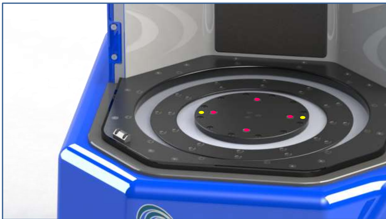
Figure 2 Resonator Plate Mounting Hole Locations LabRAM II shown without doors for illustration purposes. The doors are required for operation of the machine.
