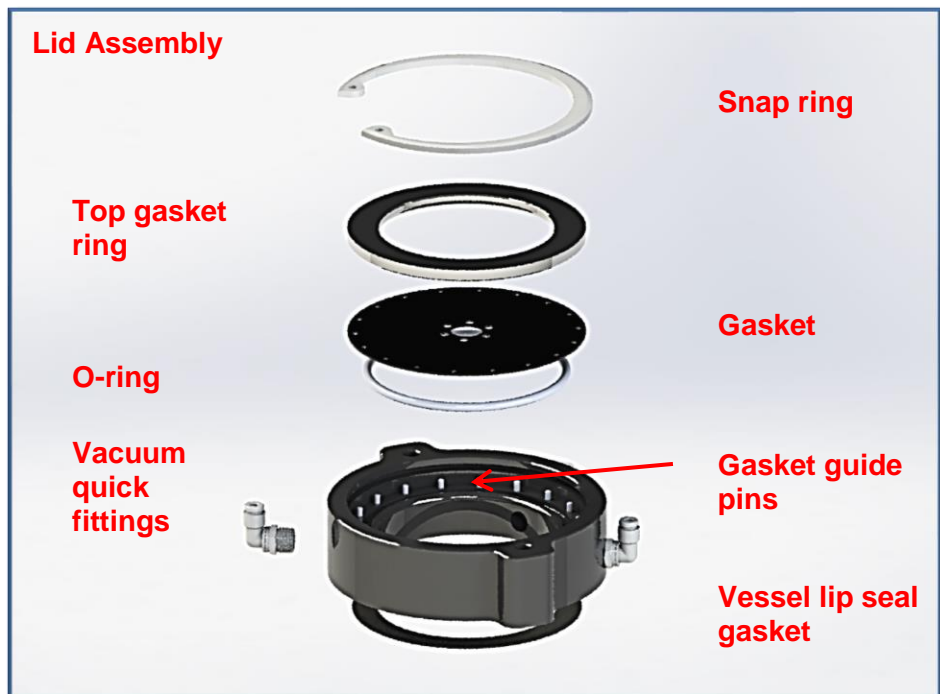
Figure 6-4: Lid Assembly Explosion (See Page 37 and 38 for Part Number listing)
