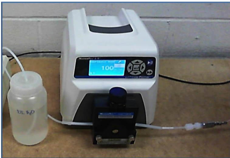
Figure 5-14: Peristaltic Pump Installation
