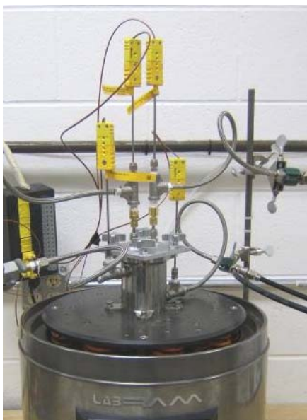
Figure 1. Instrumented Jacketed Vessel on LabRAM ® .
