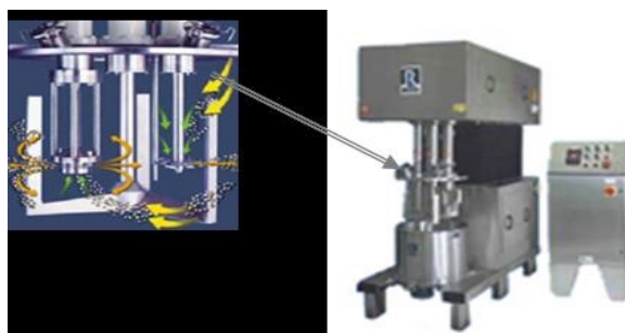
Figure 3. Multi-axis mixer required for non-Newtonian and high density mixtures.
