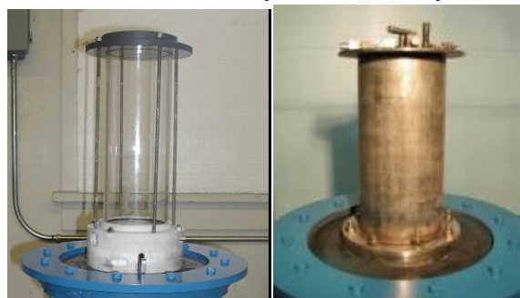
Figure 5. The ResonantAcoustic ® apparatus shown with a borosilicate glass reactor vessel on the left and a stainless steel reactor vessel on the right.
