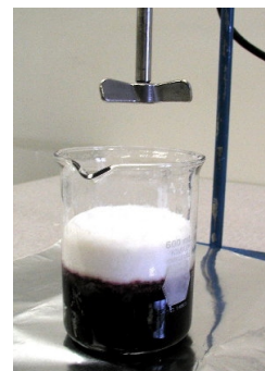
Figure 7. Conventional mixing operation using three-bladed propeller.
