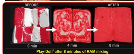
Figure 5. Mixture of Play-Doh to illustrate the mixing of two viscous liquids.
