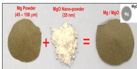
Figure 6. Micron and nano-sized particles of Mg and MgO before and after mixing. SEM micrograph of coated particle, and EDS confirmation of oxide coating.
