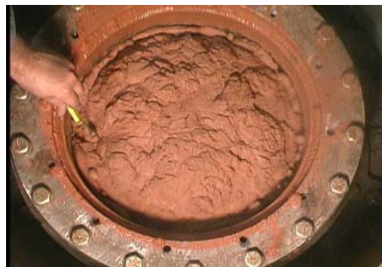
Figure 4. 120 L of Dow 200 Fluid 77% solids loaded with drywall compound and red oxide powder. Viscosity 80,000,000 cP.
