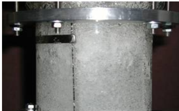
Figure 9. Gas-Liquid mixing. Air and water at 20 g acceleration.
