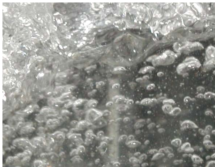
Figure 11. Close up view of gas-liquid interface at 17-g RAM acceleration.
