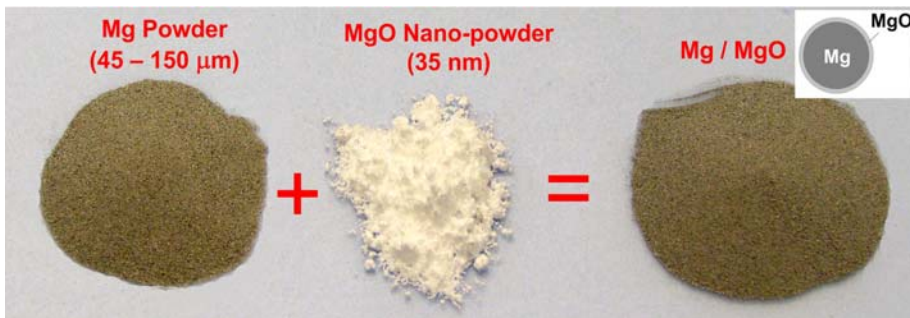
Figure 1: Appearance of micron-sized Mg powder mixed with 2 vol. % 35 nm MgO nanopowder using ResonantAcoustic® Mixing.
